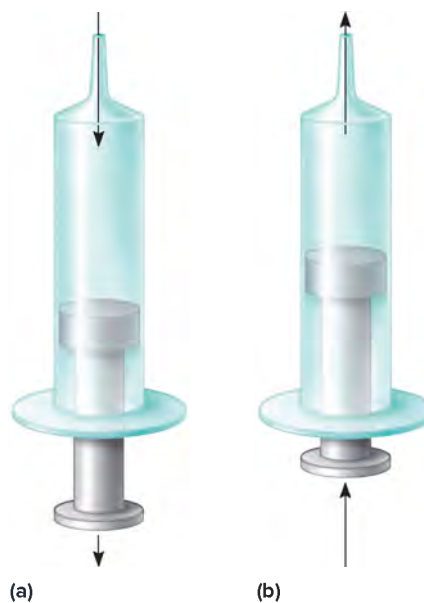
FIGURE 19.22 Moving the plunger of a syringe causes air to move (a) in or (b) out of the syringe. Air movements into and out of the lungs occur in much the same way.
