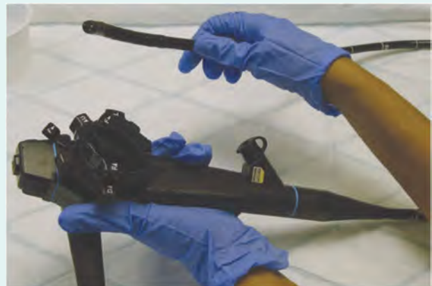
Fig. 4.72 The endoscope is a flexible plastic tube that can be controlled from the proximal end. Through a side portal various devices can be inserted, which run through the endoscope and can be used to obtain biopsies and to perform minor endoluminal surgical procedures (e.g., excision of polyps).
